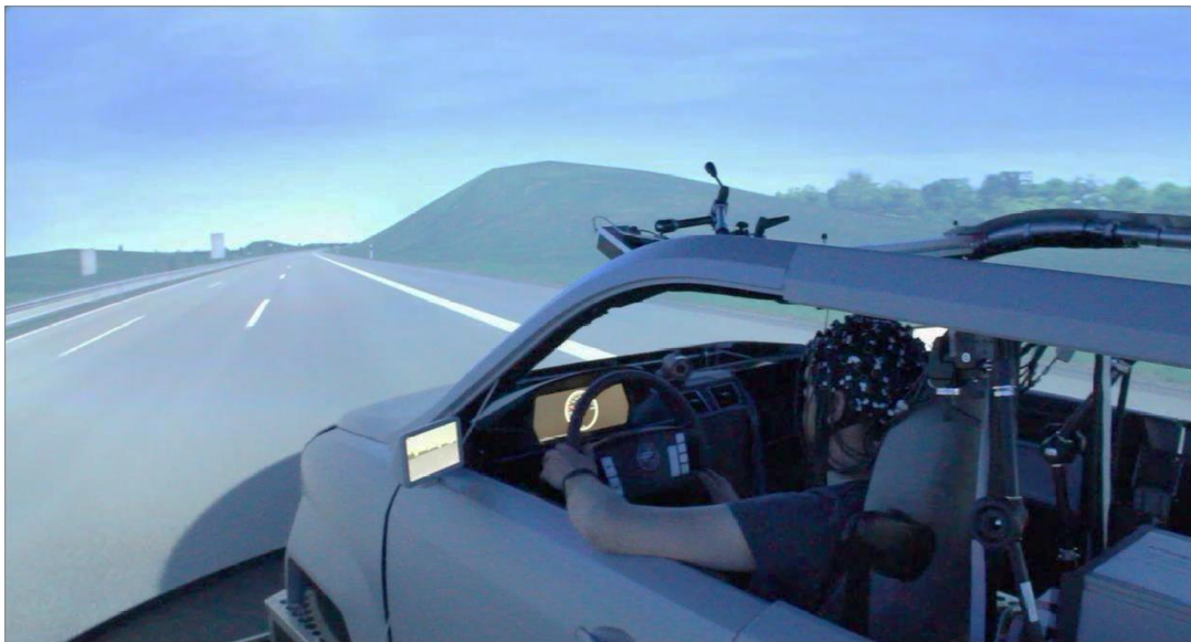
FIGURE 1 | Virtual Reality lab driving simulator at German Aerospace Center – photograph of experimental setup. The participant is driving along the highway in this experiment. The fNIRS system and the computer are positioned in the backseat of the car behind the participant (not seen in this photograph).
