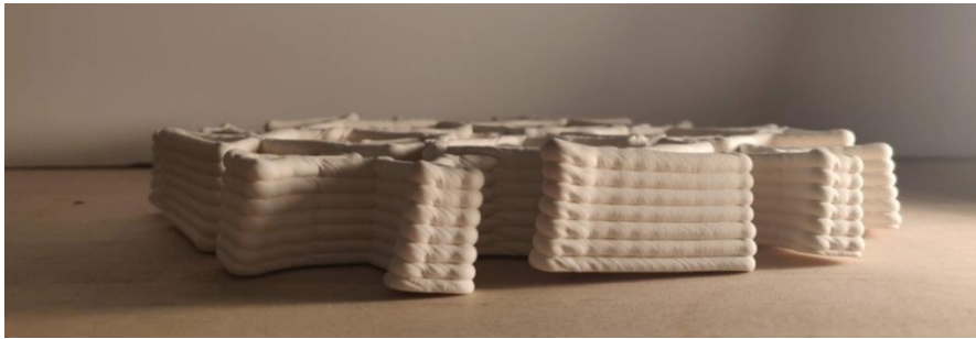
Figure 6: After firing corners of the print are lifting from the table due to warp.
