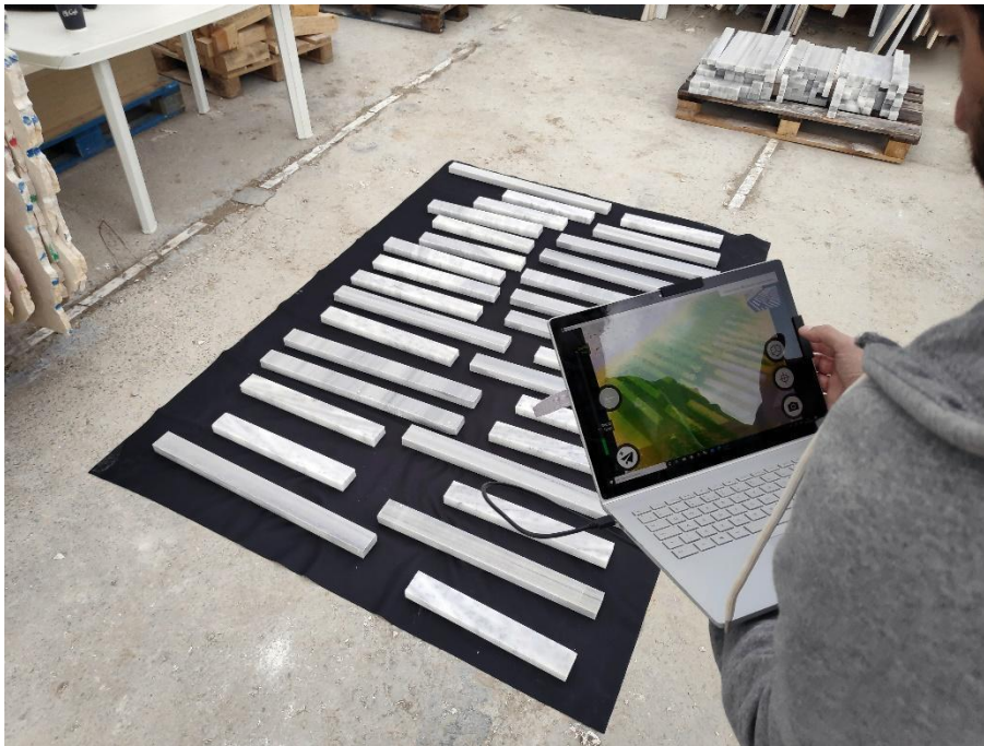
Figure 3. MABLE WEAVES 2020, marble leftover pieces registration setup
