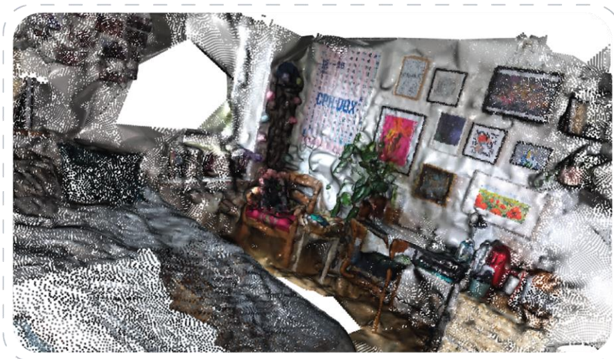
Figure 2. An example of a dense point cloud. A digital space replica of the rooms scanned for this project.
