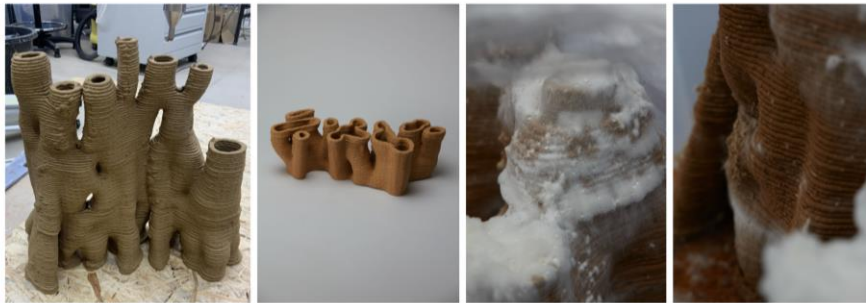
Figure 8. 3D Printed elements and mycelial growth.
