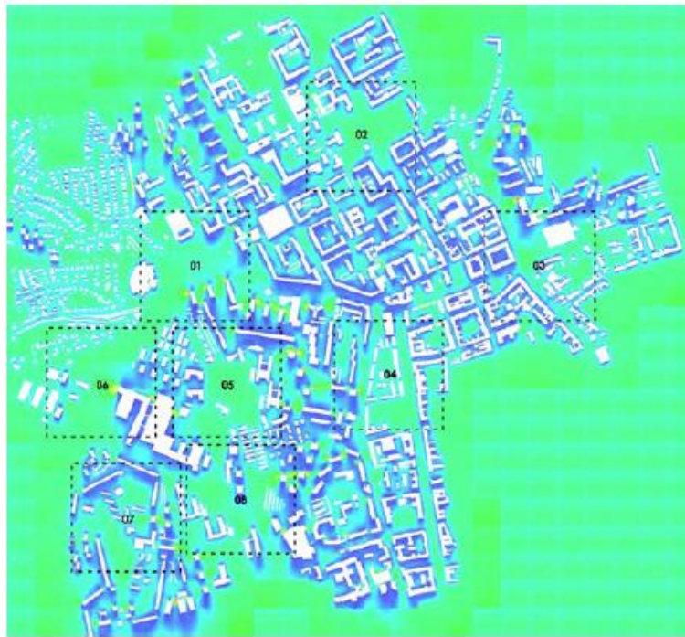
Figure 7. Wind speed prediction with InfraRed plugin. Source: Kabošová et al., 2021.
