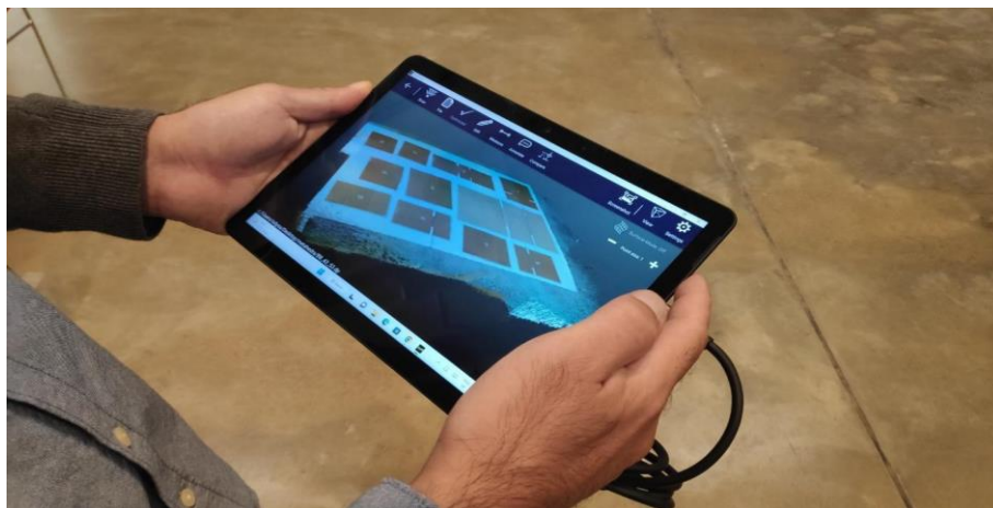
Figure 6. Capturing recyclable corrugated cardboard boxes using a Lidar Camera
