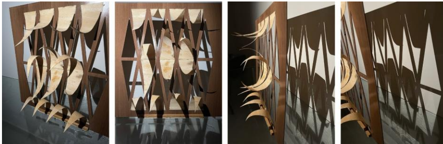
Figure 7. Patterns of deformation, light penetration, and shading effect of louvre prototype.
