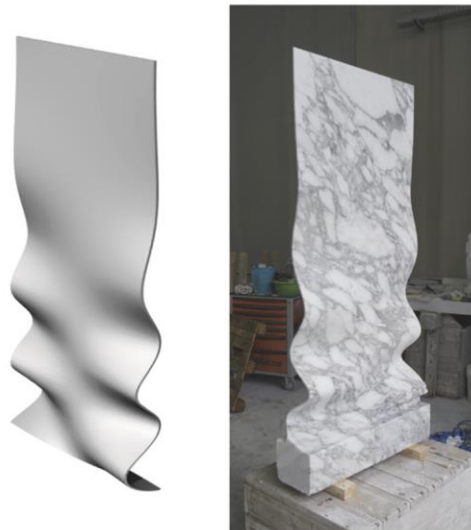
Figure 1. Digital Stone Project digital model (left), processed material (right) (Lopez, 2022).
