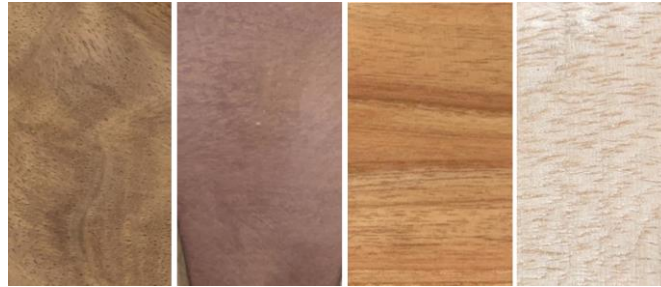
Figure 3. Local wood material samples utilized for the experiments, Left to Right: Albizia lebbeck Heartwood, Cinnamomum camphora, Melia azedarach, Albizia lebbeck sapwood.
