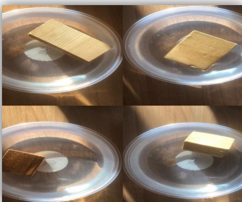
Figure.4-Wood samples inside the containers filled with water Source: Authors
