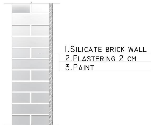
Fig. 6 – Building B masonry, CAD, Source: Authors.
