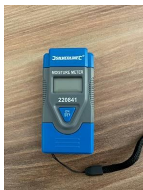
Fig. 10. Silverline Digital Moisture Meter. (Source: Authors).
