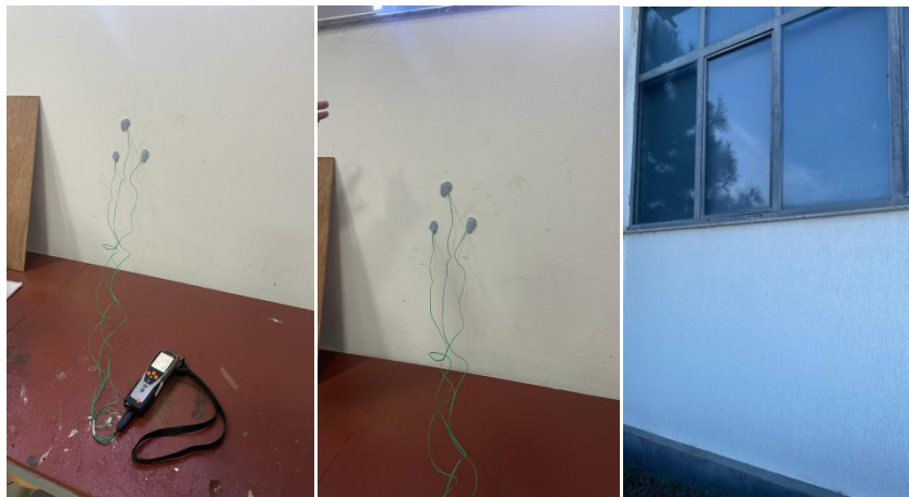
Figure 5. A. Testo 435-2 measurement device during second measurements. B. Internal sensors C. Position of external wireless sensor; source: author
