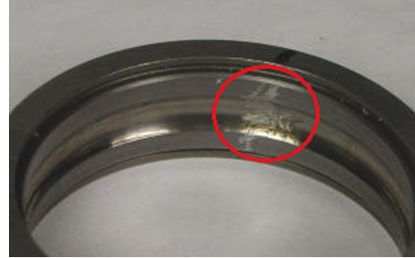
FIGURE 8: A photo of outer race fault.
