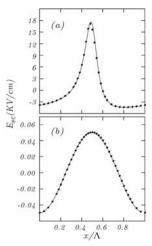
Fig. 2. Space-charge field as function of the modulation with: a) m=0.9,  $\wedge = 1.0$  and b) m=0.01,  $\wedge = 20.0$ . The dotted line is the result of numerical solutions and the continuous line is the result for analytical function.
