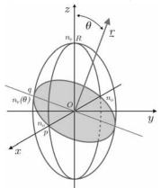
Fig.3. Normal modes determined from the Index ellipsoid.
