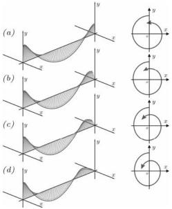
Fig.9. Evolution of the plane of polarization as function of the applied field for: a) 50V. b)200V. c)400V and d)600V.
