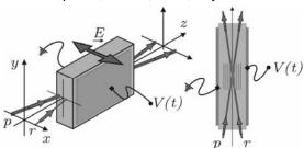
Fig. 5. Schematic of the experiment for two-wave mixing.
